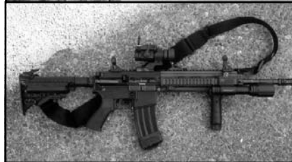
The 14.5” HK 416 upper receiver carbine with Troy Industries BUIS, Aimpoint, plus LaRue mount and Battle Light.
