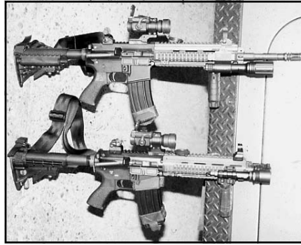
HK 416 upper receivers on RRA lowers. Top, 14.5", bottom 10" version used in test.
