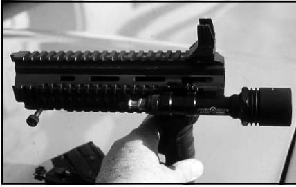
HK 416 unique design free-floating Picatinny rail forearm: easy on and off with no change in zero.
